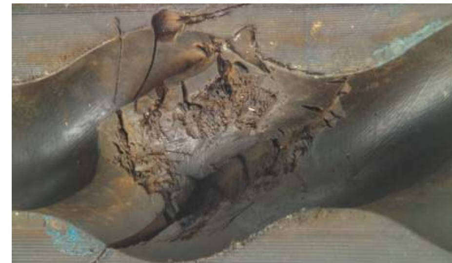
Cheap copy: Failed after short time operation due to delamination of stator parts.
