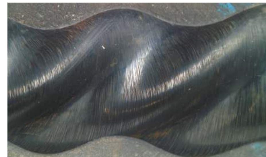
Original: Virtually no signs of wear under the same operating conditions.
