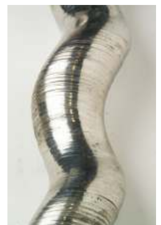
Cheap copy: Rotor made of an unknown metal with high wear and poor efficiency.
