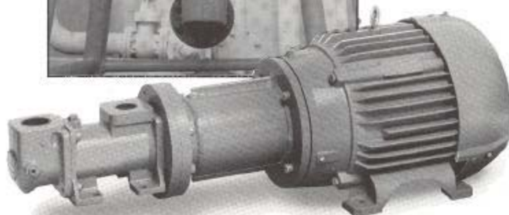
Model A3D with 15 hp magnetic drive and TEFC motor, 15 gpm, 300 psig discharge, 9600 SSU, 1200 rpm. Horizontal foot mounted.
